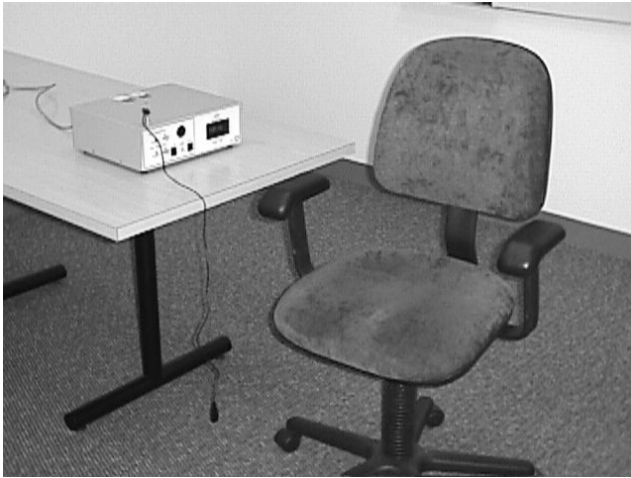
Figure 3. Test Setup to Measure Number of ESD Events
